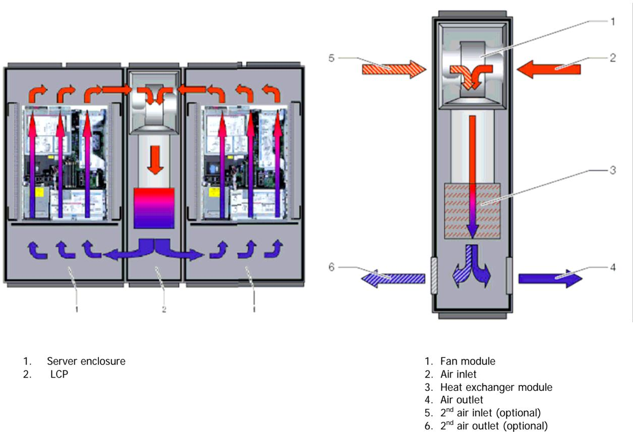
Figure 2: Top view of air inlet/outlet paths
