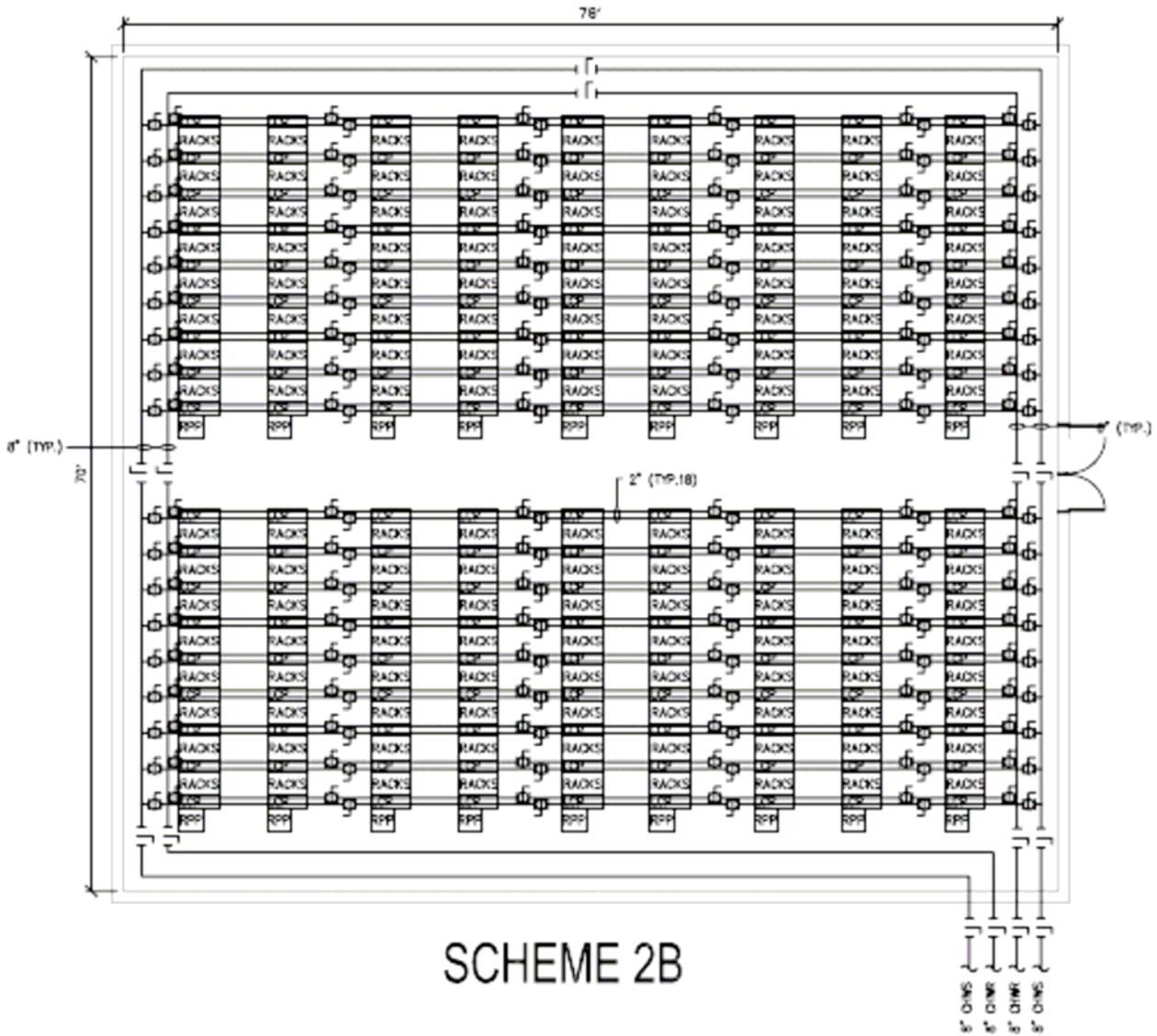
Figure 7: Layout of LCP 5,500 ft<sup>2</sup> data center
