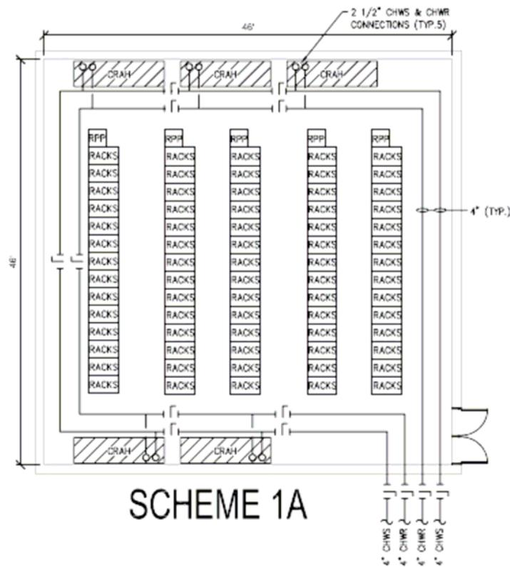
Figure 4: Layout of Legacy 2,100 ft<sup>2</sup> data center
