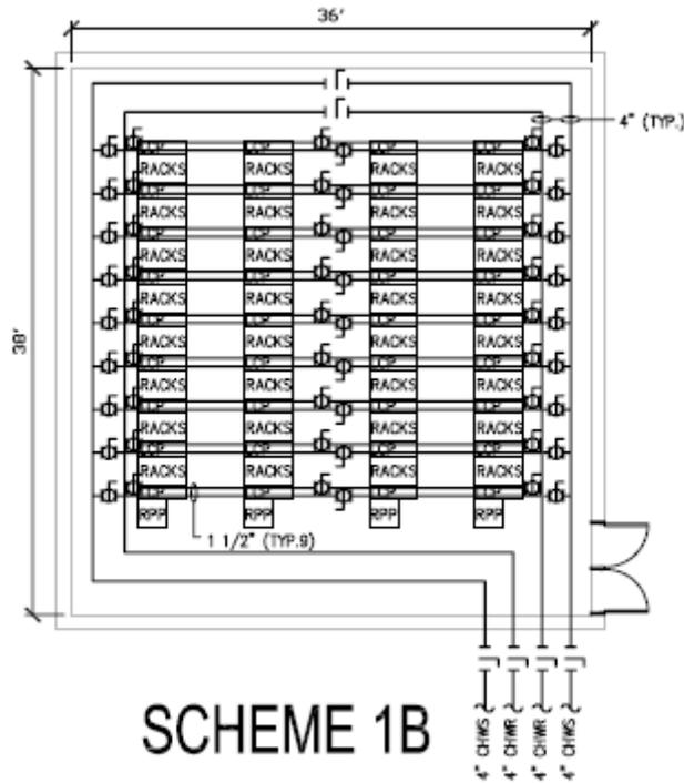
Figure 5: Layout of LCP 1,400 ft<sup>2</sup> data center
